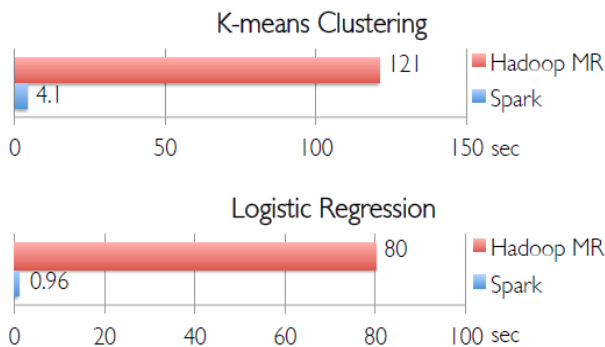
Fig 5. Two Iterative Machine Learning Algorithms
