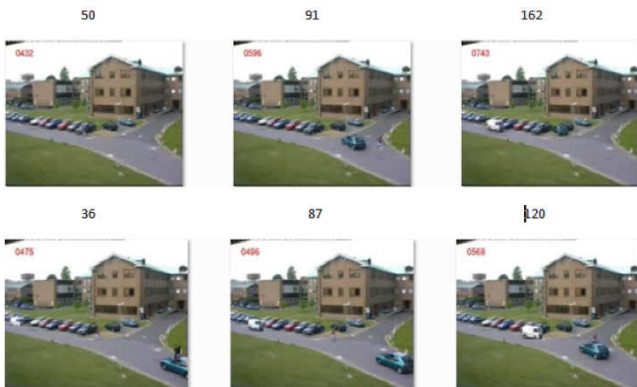
Figure 5.1: Surveillance video; First row shows video synopsis of frame based method [8], second row shows a result obtained by combining frame based and object movement based video synopsis.
