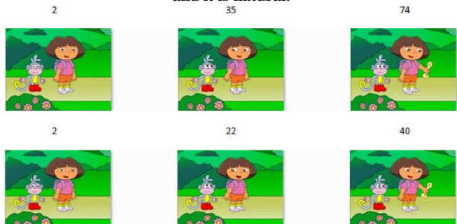
Figure 5.4: Cartoon: Adventure of Dora and Buji; First row represents the object based method [2], Dora and Buji speak together, it is not realistic. Second row shows object movement based video synopsis each object separately to produce a synopsis [2], and preserve the chronological order of speakers.
