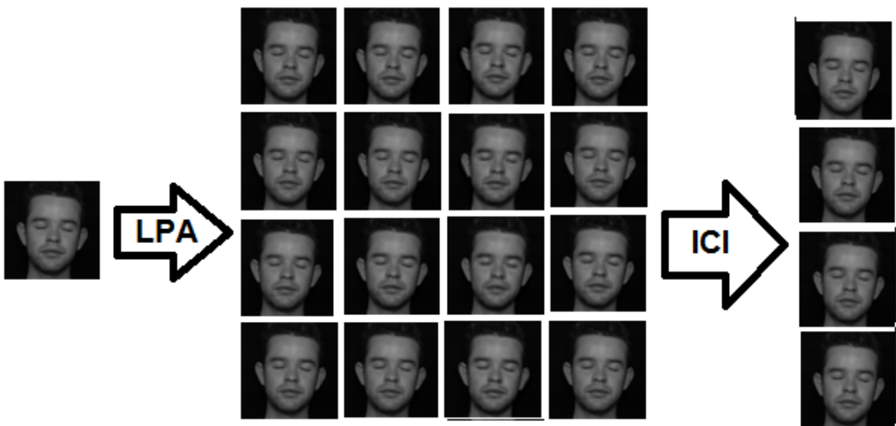
Figure 2. The face image is convolved with LPA filters to get directional faces.Optimised using ICI in each direction to obtain Optimised Directional Face in each direction
