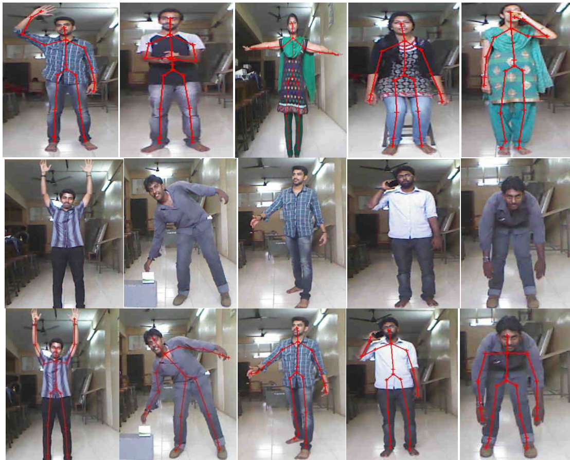
Fig. 8: Sample images from videos of the 10 activities in our database. We show RGB image frames as well as the corresponding skeleton joint positions. Action type from left to right, top to bottom: high arm wave, clap hands, hand wave, sit down, dinking, hands up, pick up, walk, phone call, bend.
