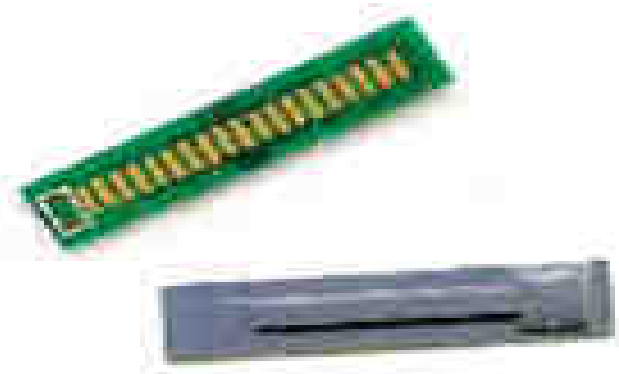
Fig. 2.9(a) AT77C104B Finger Chip IC.
