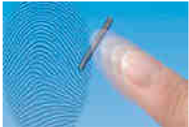
Figure 2.9(b) Typical fingerprint—and finger being swept over a sensor.
