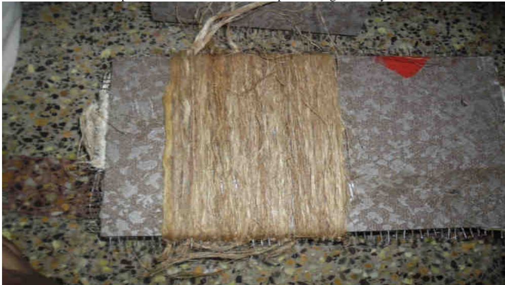
Fig. 1 – Preparation of unidirectional Jute and Banana fiber composites
