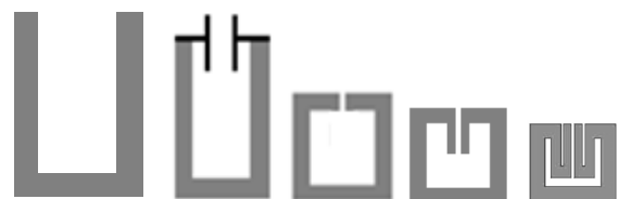
Fig. 1. Actual, capacitor loaded, single-fold, double-fold and four-fold resonators
