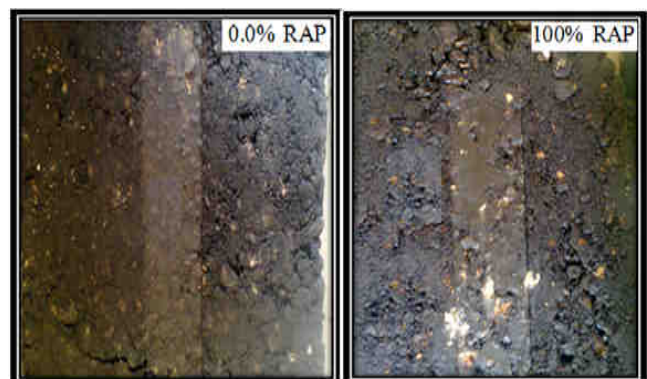
Fig. 14 Rutting depths after track wheel test
