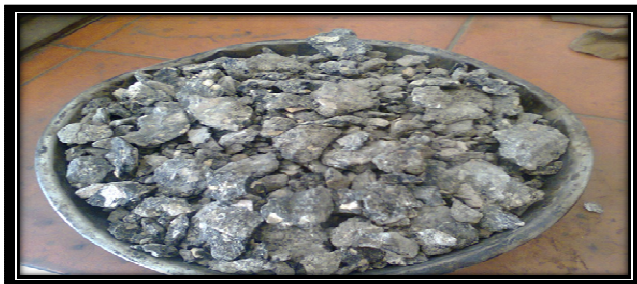
Fig. 2 Reclaimed asphalt pavement
