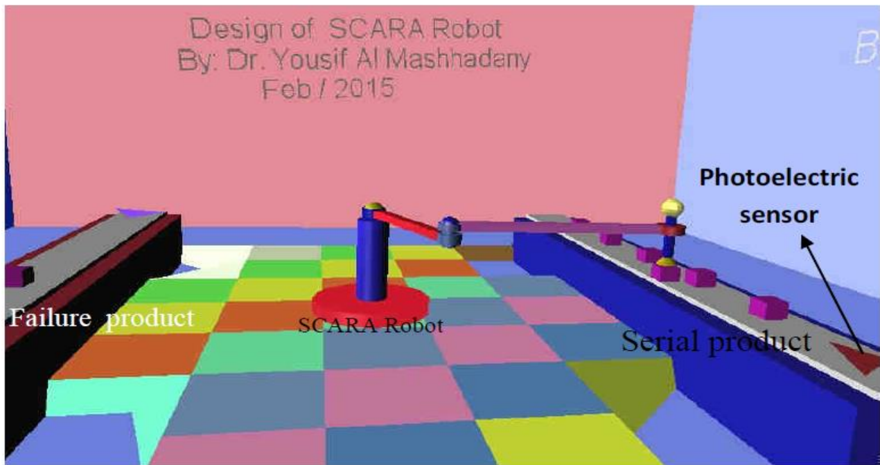
Fig.3. A SCARA robot left arm, in VR view through Matlab
