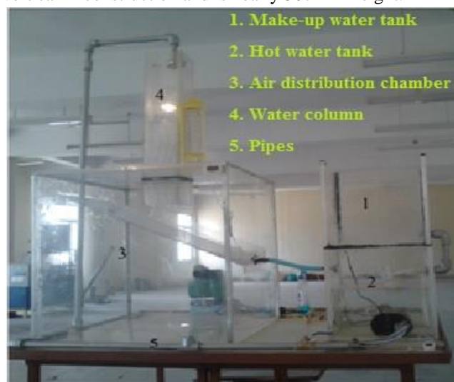
Fig. 4: Model of fabricated cooling tower
