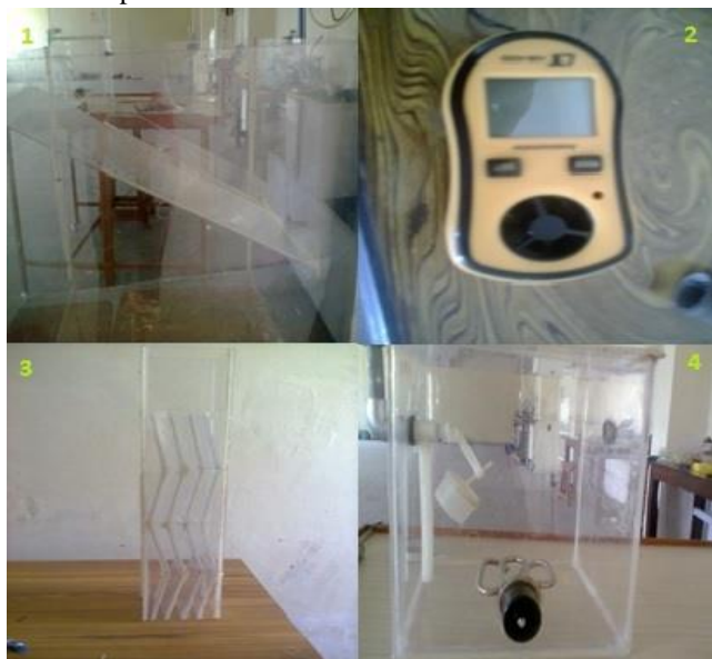
Fig. 3: Water collecting basin, Anemometer, Water column, Hot water tank
