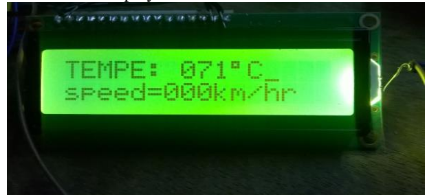
Fig.4 Real Time Temperature
