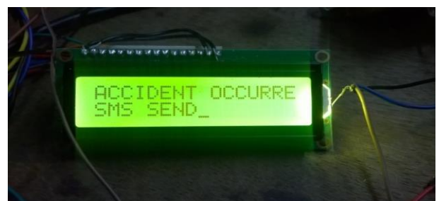
Fig.7 Accident Detection and SMS alert
