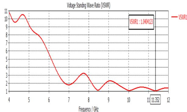
**Figure.7: VSWR of proposed antenna at frequency  $f=11.352$ GHz**
