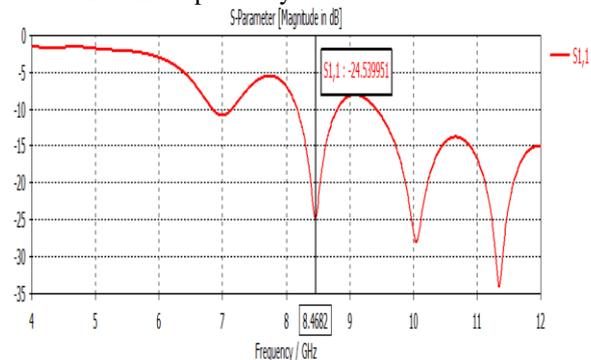
**Figure.2: Return loss of proposed antenna at frequency f=8.4682GHz**
