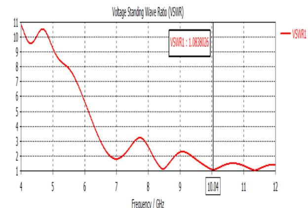
**Figure.6: VSWR of proposed antenna at frequency  $f=10.04$ GHz**
