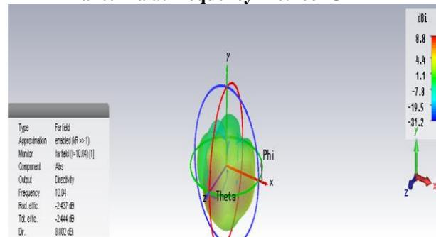
**Figure.9: 3-D plot of far field pattern of proposed antenna at frequency  $f=10.04$ GHz**
