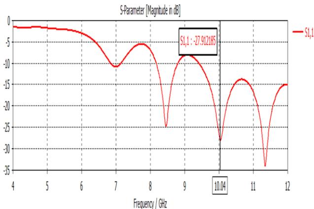
**Figure.3: Return loss of proposed antenna at frequency  $f=10.04$  GHz**
