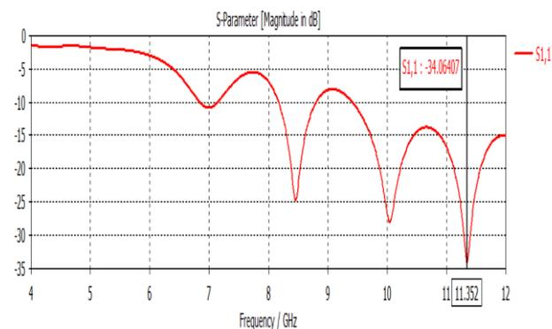
**Figure.4: Return loss of proposed antenna at frequency  $f=11.352$  GHz**
