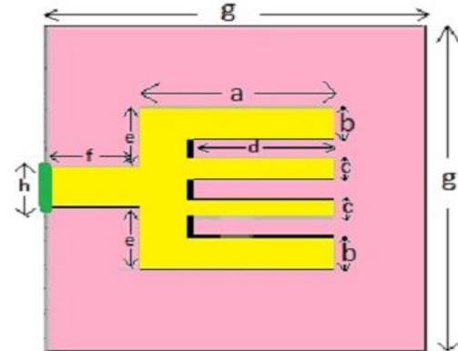
**Fig.1: Fork shaped microstrip antenna**
