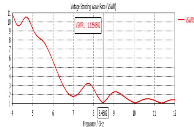
**Figure.5: VSWR of proposed antenna at frequency  $f=8.8462$ GHz**
