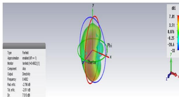
**Figure.8: 3-D plot of far field pattern of proposed antenna at frequency  $f=8.4682$ GHz**
