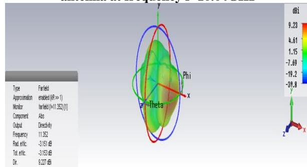
**Figure.10: 3D plot of far field pattern of proposed antenna at frequency  $f=11.352$ GHz**
