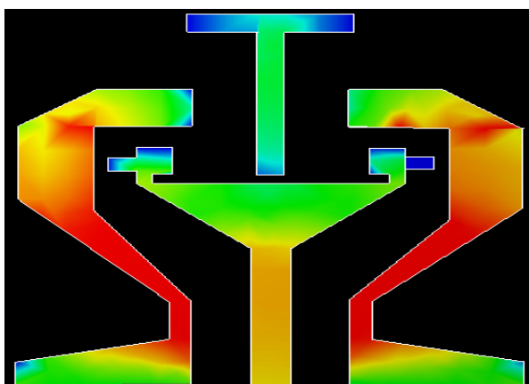
Figure. 6 (c) Surface Current Distribution at 6.4 GHz
