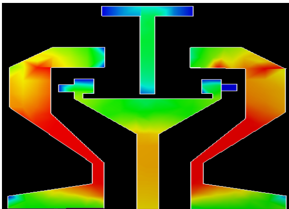
Figure. 6 (c) Surface Current Distribution at 6.4 GHz
