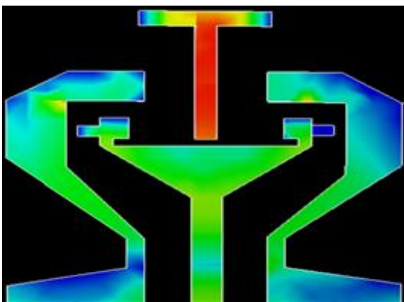
Figure. 6 (b) Surface Current Distribution at 5.5 GHz
