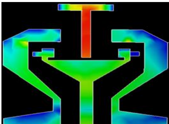
Figure. 6 (b) Surface Current Distribution at 5.5 GHz
