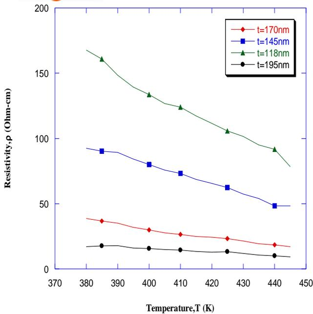
Fig.8. Variation of Resistivity with Temperature for CoS thin films.
