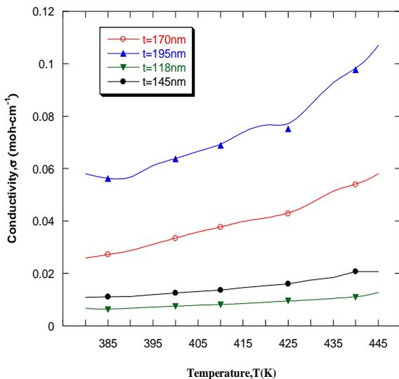
Fig.9. Variation of conductivity with temperature for CoS thin films
