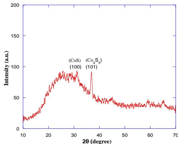
Fig. 2. XRD patterns of cobalt sulfide thin films
