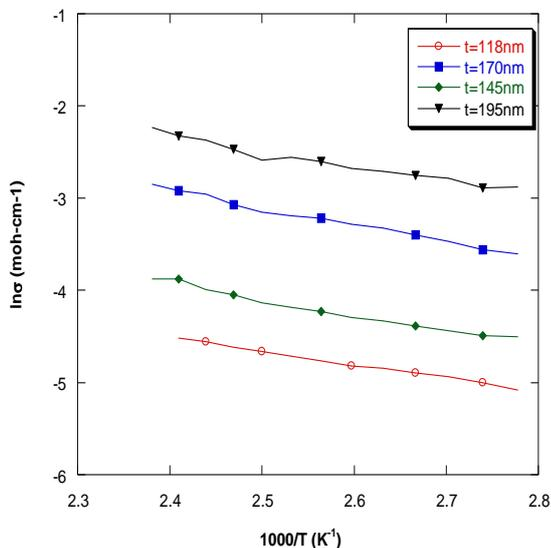
Fig.10. Variation of  $\ln\sigma$  with  $(1/T)$  inverse temperature for CoS thin films.
