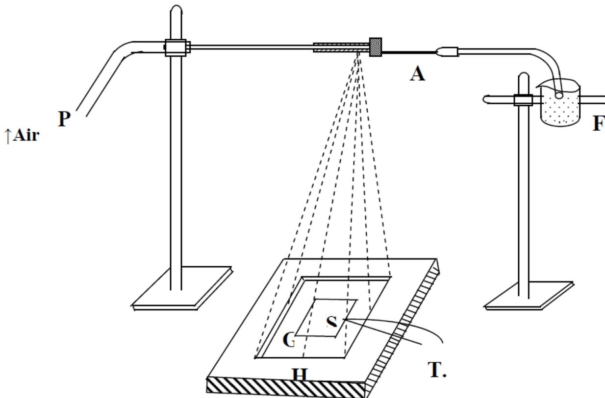
A - Lower tube, G - Steel plate, H - Heater S = Substrate, P = Compressed air (Upper tube) T. C. = thermocouple F = chemical solution (Beaker)
