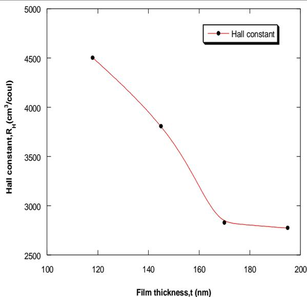
Fig.5. Variation of Hall constant( $R_H$ ) with thickness(t) for CoS thin films.
