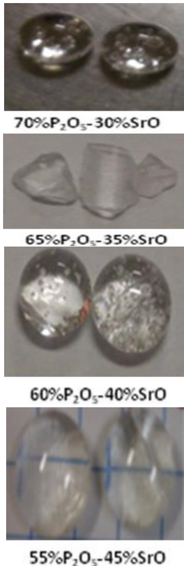
Figure 2: Photograph image of glasses \text{P}_2\text{O}_5\text{-SrO}
