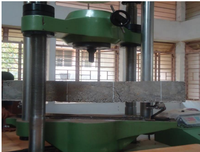
Fig. 4.2 Failure of Beam N-CB1
