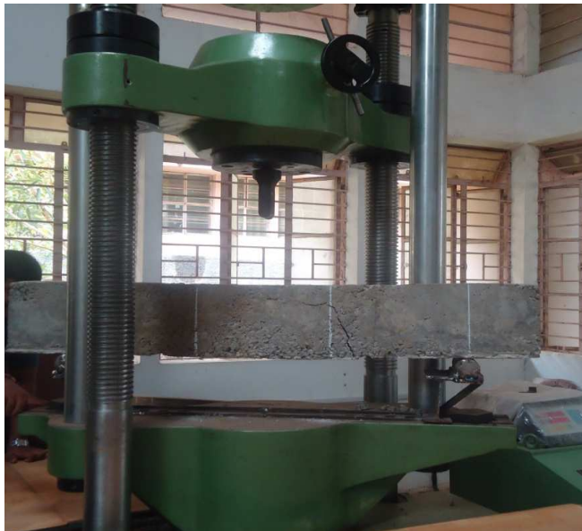
Fig. 4.2 Failure of Beam N-CB1
