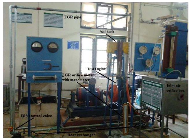
Fig. 5: Exhaust Gas Recirculation Setup
