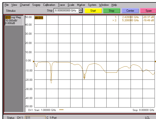
Figure 4 Return Loss of Antenna (Hardware Results)
