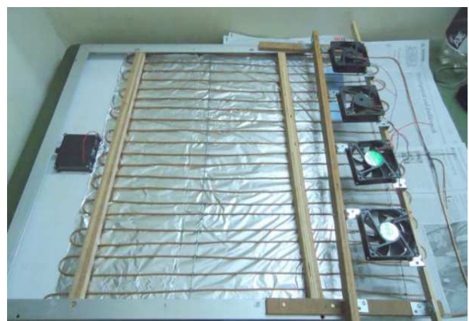
Fig. 5 Pulsating Cooling Pipe Arrangement on the Rear Side of PV Panel
