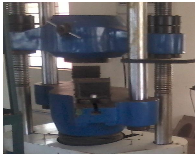
Figure 2. Compressive Strength Test in UTM
