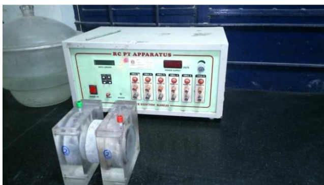
Figure 3. Rapid Chloride Permeability Test Apparatus Table 3 Rating of Chloride ion Penetrability Based on Charge Passed as per ASTM C1202
