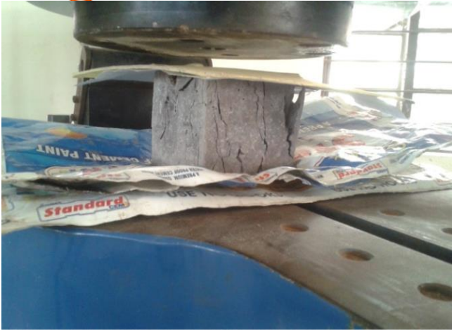
Figure 5. Crushed Specimen After Completion of Compressive Strength Test
