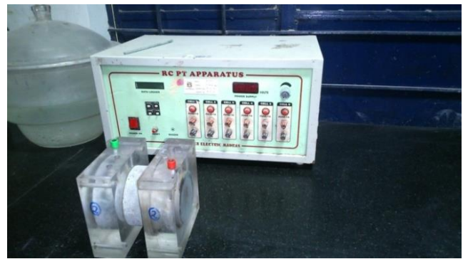
Figure 3. Rapid Chloride Permeability Test Apparatus
