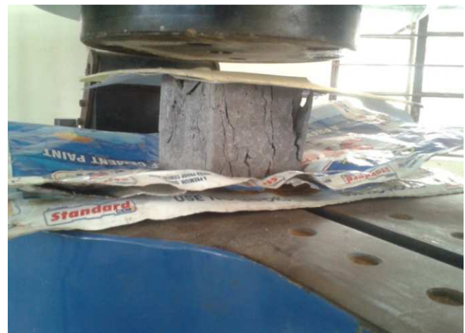
Figure 5. Crushed Specimen After Completion of Compressive Strength Test
