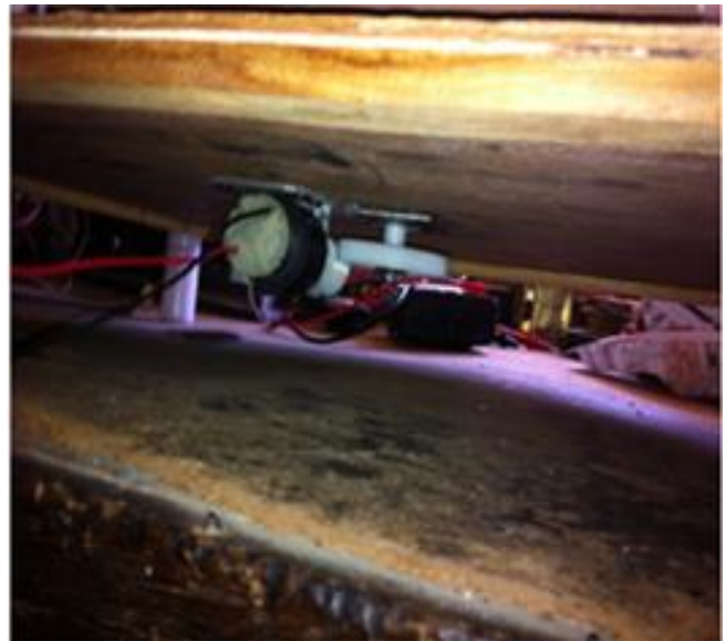
Fig 6: Horizontal Motor Terminal with Side Shaft Gear
