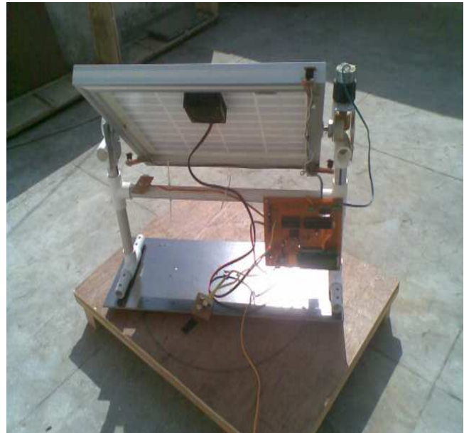
Fig 10: PCB connection with solar panel
