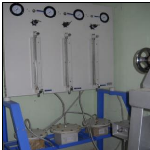
Fig. 2(b) – Parts of Permeability Machine showing pressure dials, valves, water columns and installed assembly of
