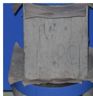
Fig. 1 – Sample at failure.
