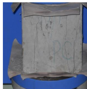
Fig. 1 – Sample at failure.
