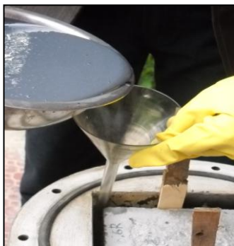
Fig. 2(c) – Sealing of sample using Epoxy sealant.
