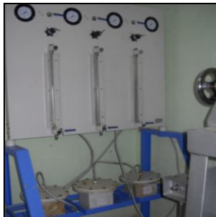
Fig. 2(b) – Parts of Permeability Machine showing pressure dials, valves, water columns and installed assembly of samples.
