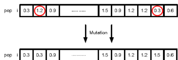
Figure 4. A sample mutation operation
