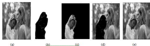
Fig.8 (a) Pair Image (b) Edge Map of Low resolution image ROI (c) Lossless Compression to ROI of Low resolution image (d) Lossy Compression for background (e) Final Compressed image of Low resolution image
