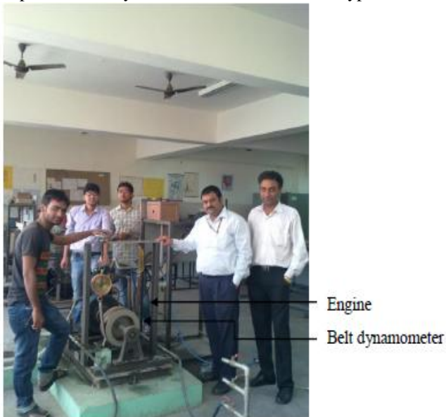
Fig.-7. Engine with dynamometer arrangement
