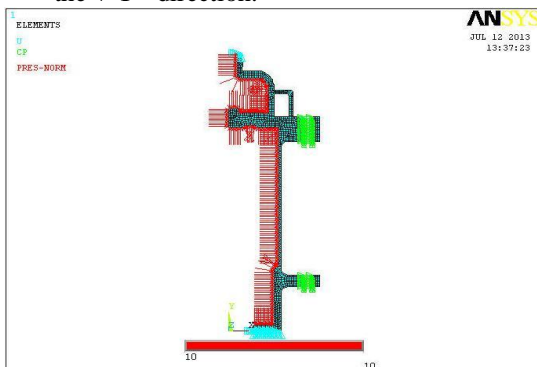
Figure 7.1: Thruster mesh with boundary conditions
