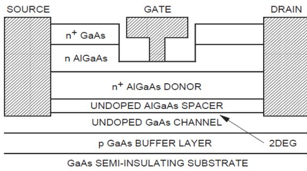
Figure.1. AlGaAs/GaAs HEMT Structure [2]
