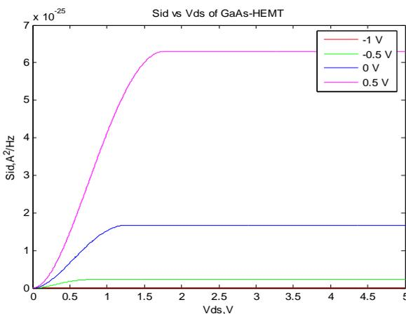
Figure.6. Plot for Sid vs. Vds of GaAs-HEMT for  $V_{gs}=-1,-0.5, 0, 0.5$  V, over the range of  $V_{ds}=0$  to 5 V (at step size of 0.5 V) [1, 19].
