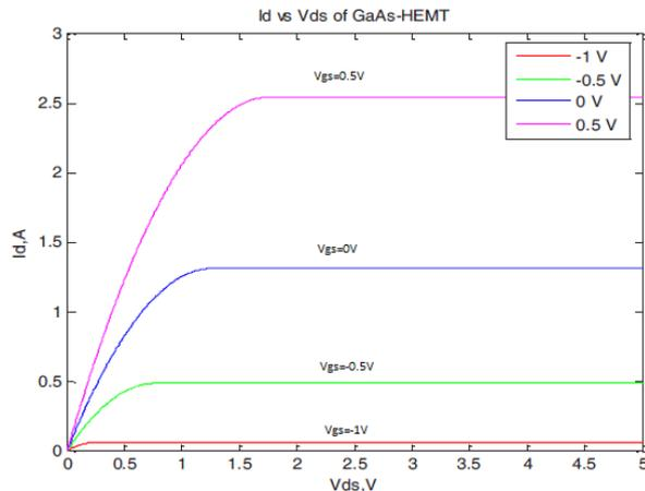
Figure.4. Plot for I-V characteristics of GaAs HEMT for  $V_{gs} = -1, -0.5, 0, 0.5 \text{ V}$ , over the range of  $V_{ds} = 0$  to 5 V (at step size of 0.5 V) [1].
