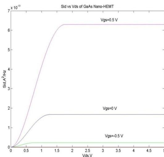
Figure.7. Plot for Sid vs. Vds of GaAs Nano-HEMT with  $L_g=1$  nm for  $V_{gs}=-1,-0.5, 0, 0.5$  V, over the range of  $V_{ds}=0$  to 5 V (at step size of 0.5 V)
