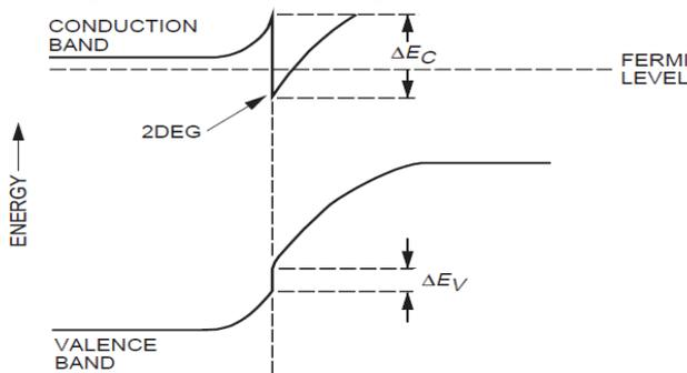
Figure.2. Energy band diagram of a generic AlGaAs–GaAs HEMT showing the 2D Electron Gas quantum well channel [2].
