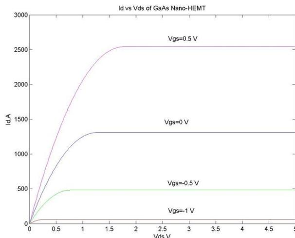
Figure.5. Plot for I-V characteristics of GaAs Nano-HEMT with  $L_g = 1 \text{ nm}$ , for  $V_{gs} = -1, -0.5, 0, 0.5 \text{ V}$ , over the range of  $V_{ds} = 0$  to 5 V (at step size of 0.5 V).
