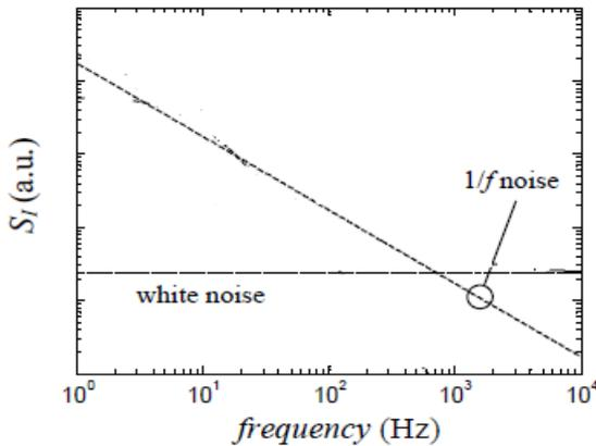
Figure.3. Nature of typical characteristics of  $1/f$  noise involved with the semiconductor devices over a range of frequency<sup>[17]</sup>.
