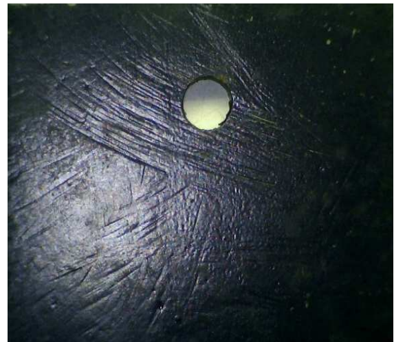
Fig 4.2 Image of Teflon coated after 168 hrs. salt immersion test.
