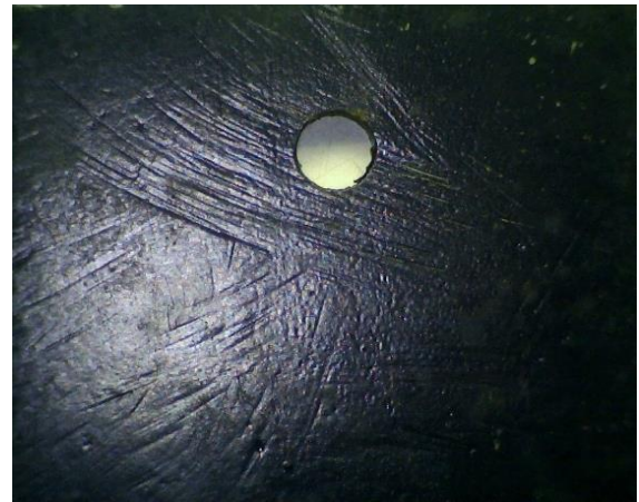
Fig 4.2 Image of Teflon coated after 168 hrs. salt immersion test.
