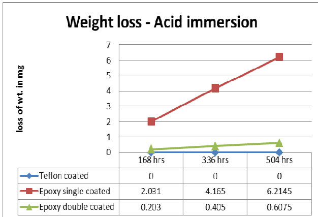
Fig 4.5 Weight loss comparison after acid immersion test
