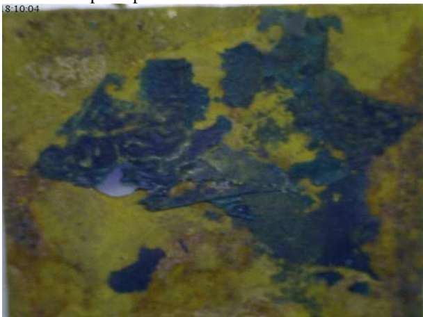
Fig 4.3(c) Image of epoxy single coated after 168 hrs acid immersion test
