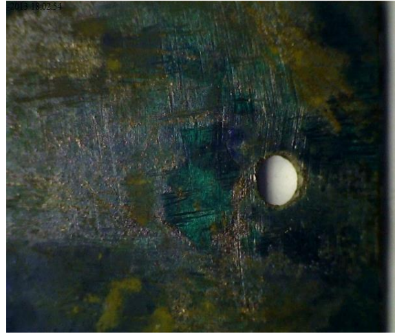
Fig 4.1(b) Image of epoxy coated after 168hrs. salt immersion test.
