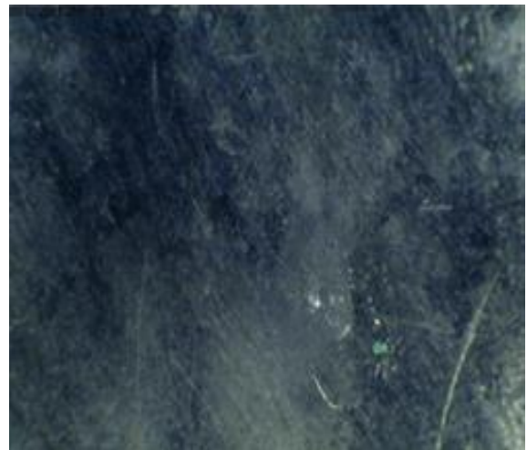
Fig 4.3(a) Image Teflon coated after 168 hrs acid immersion test
