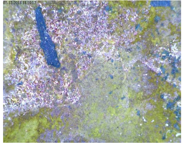
Fig 4.3(d) Image of epoxy single coated after 168 hrs acid immersion test(scale X200)
