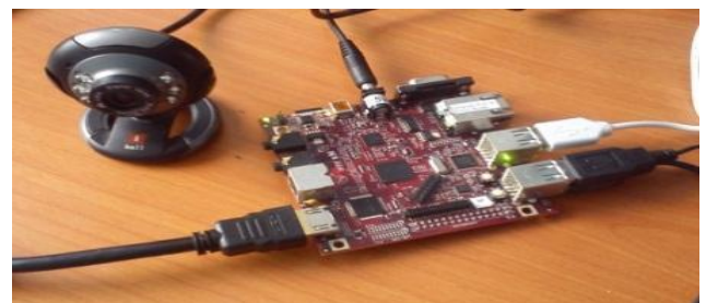
Fig 1. Experimental setup with BeagleBoard and web camera
