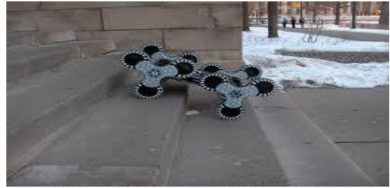
Fig.4 Tri-lobe wheel stair climber
