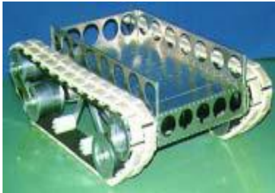
Fig.2 Tracked (belt & chain) type
