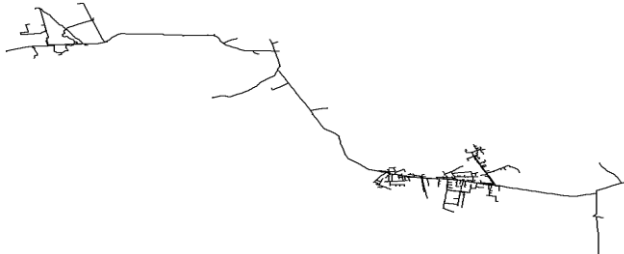
Figure 2: Single-line diagram of actual power network of Kosar feeder of Kerman Province in Cymedist
