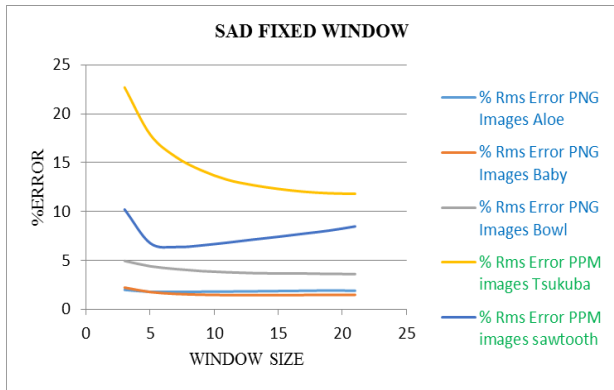
Fig.6 Evaluation of SAD Algorithm: Window size vs % Error for PNG and PPM images
