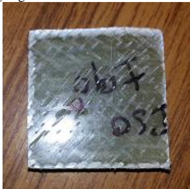
Fig.4 Specimen prepared for Burning Test
