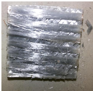
Fig.5 Specimen after Burning Test (GP)
