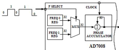
The AD7008 has three registers that can be used for modulation. Besides the example of frequency modulation shown above, the frequency registers can be updated dynamically as can the phase register and the IQMOD register. These can be modulated at rates up to 16.5 MHz. The example shown below along with code fragment shows how to implement the AD7008 in an amplitude modulation scheme. Other modulation schemes can be implemented in a similar fashion.
