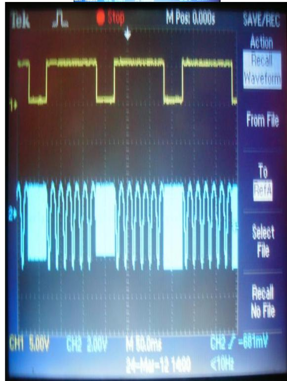
The above snap shot shows the output of the system as frequency synthesizer. The frequency entered through the keyboard is displayed on CRO.
