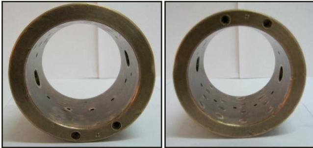
Figure 4: (a) Smooth bearing, (b) Textured bearing
