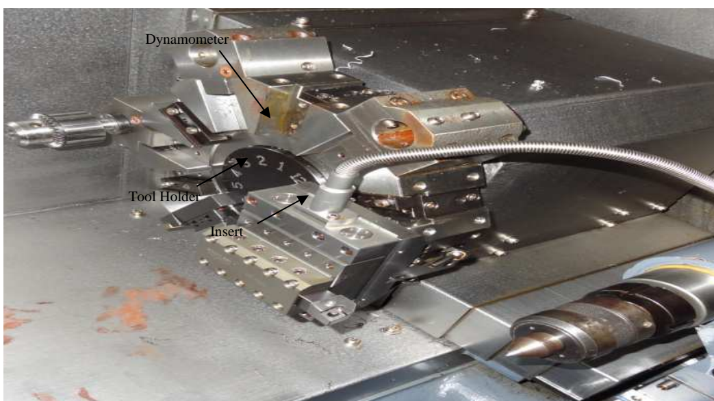
Figure1. Tool insert and piezoelectric dynamometer in CNC lathe machine
