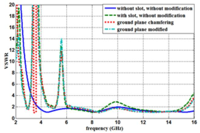
Fig.4. Simulated VSWR of the proposed antenna.
