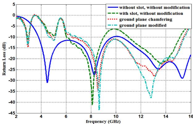
Fig.3. Return loss of the proposed antenna.
