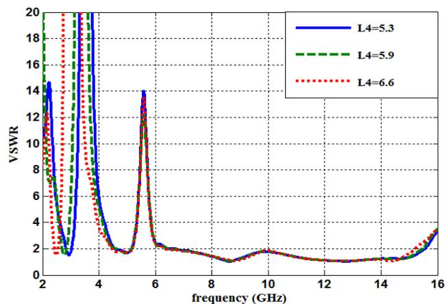
Fig. 9 Effects of the varying the length  $L_4$  of the symmetrical L-slot on the notched bandwidth 3-4 GHz.
