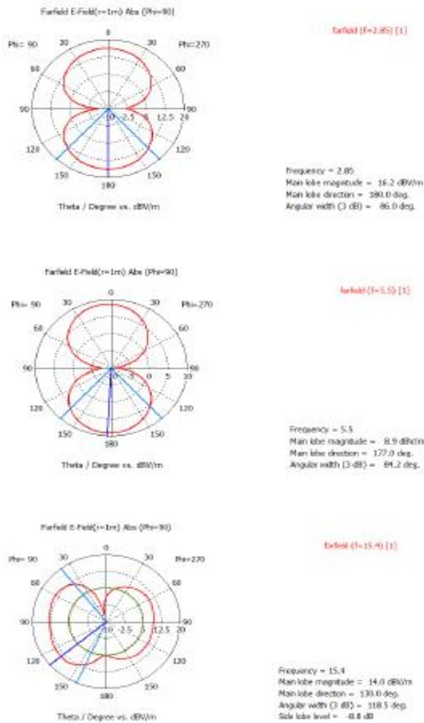
Fig.11. Polar plot of far-field antenna pattern at selected frequencies in the y-z plane
