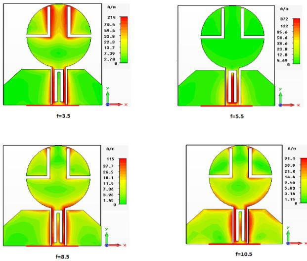
Fig.10. Current distribution at 3.5 GHz, 5.5 GHz, 8.5 GHz and 10.5 GHz.
