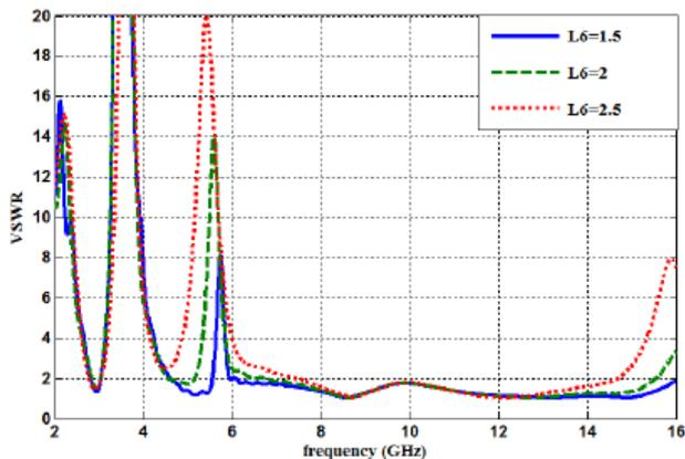
Fig.6. Effects of the varying the length  $L_6$  of the inverted U-slot on the notched bandwidth 5-6 GHz.
