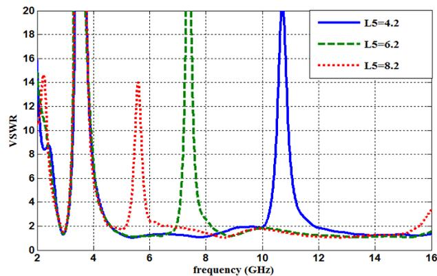
Fig.7. Effects of varying the length  $L_5$  of the inverted U-slot on the notched bandwidth 5-6 GHz.
