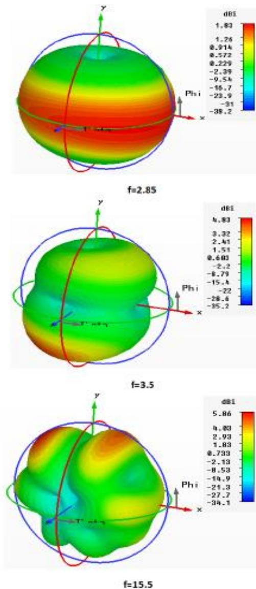
Fig.12. 3D plot of field pattern shows the gain at selected frequency.
