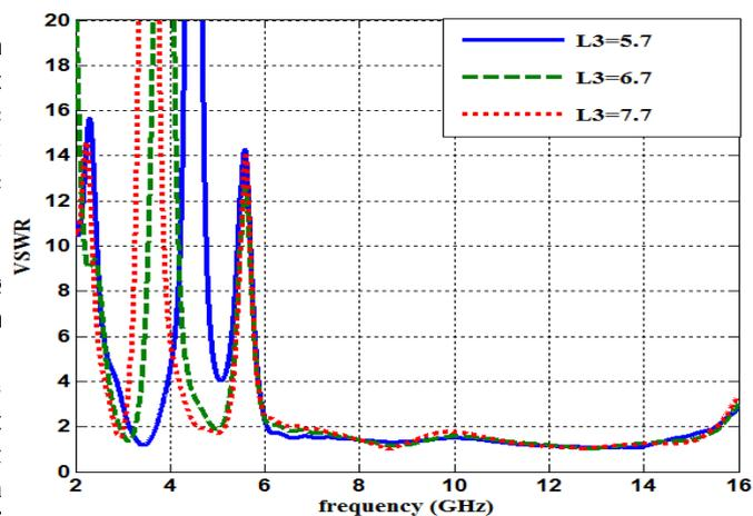
Fig.8. Effects of varying the length  $L_3$  of L-slot on the notched bandwidth 3-4 GHz.
