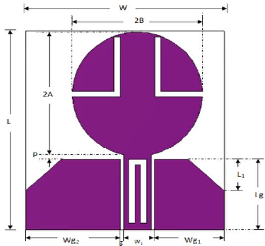
Fig. 1 Geometry of proposed dual-band notched UWB antenna.
