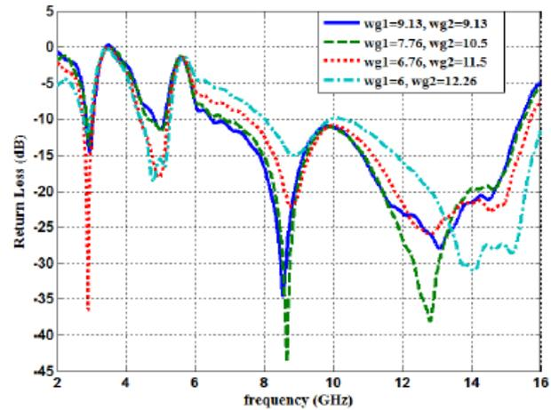
Fig.5 The return loss responses of modeled printed elliptical monopole antenna with different width  $wg_1, wg_2$ .
