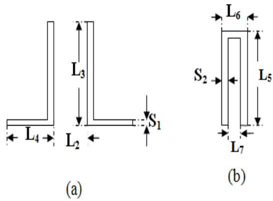
Fig. 2 Configuration of proposed cutting slot (a)symmetrical L-shape (b) inverted U-shape.
