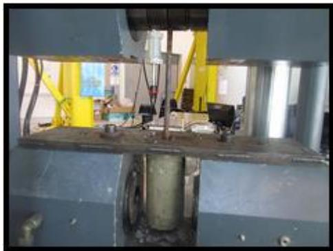
Figure 6 Test Set up for Pull out Test
