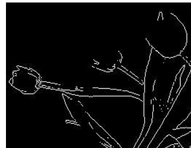
Fig. III.3.4 Edgeextracted by Sobel operator
