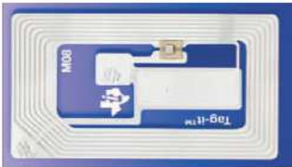
Figure-3. Tag-it HF-I plus transponder (RI-I03 112A-03)
