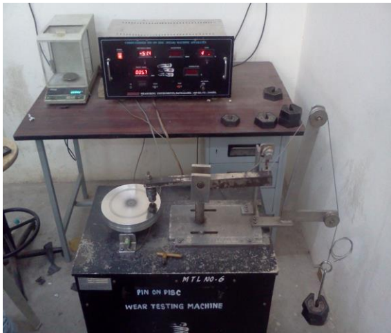
Fig 3: Pin on disc setup
