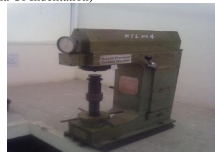
Fig 2: Brinell hardness testing setup
