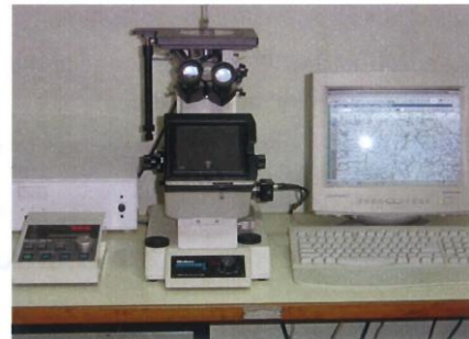
Figure 4.5 Versamet optical microscope with clemex image analyzing system
