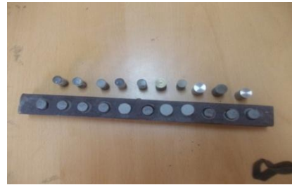
Figure 4.4 90% Al + 10% Al 2 O 3 coating produced over A356 substrates
