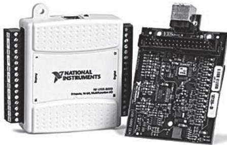
Figure16. Data acquisition card USB 6009
