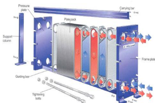
Fig. 1 Gasket plate heat exchanger assemblage and parts
