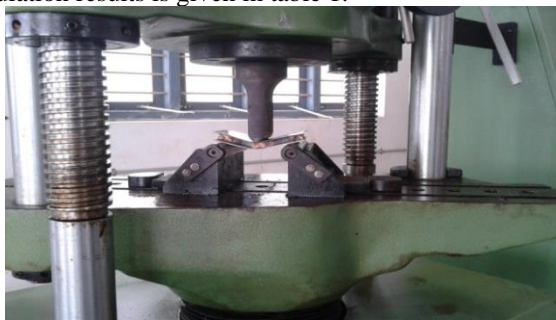
Figure 6: Specimen loaded and tested using UTM
