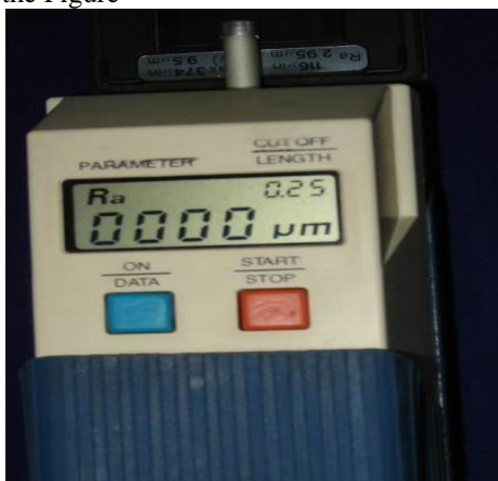
Fig: Mitutoyo Tally Surf Tester
