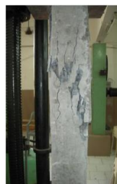
Fig. 4: Failure Pattern of Column Element CE
