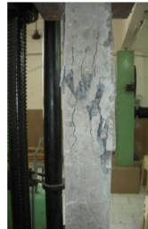
Fig. 4: Failure Pattern of Column Element CE
