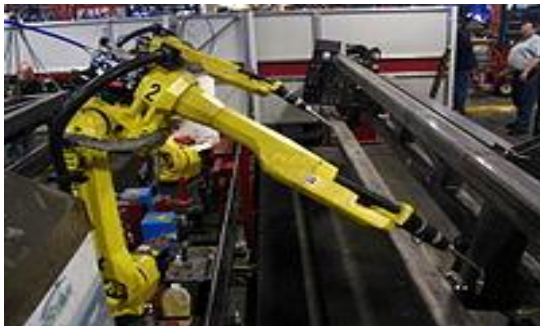
Fig 2: Articulated Welding Robots used in a Factory [1]
