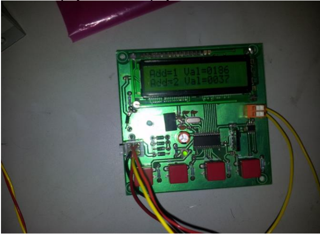
Fig 11: Results of Pressure and Thermocouple Analog Card
