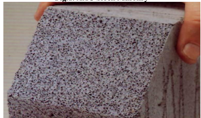
Fig.2-Porous structure of AAC block
